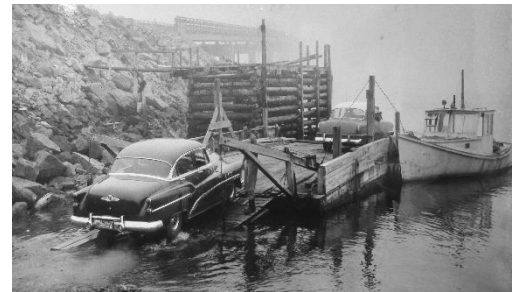
Automobile ferry service began in 1951 and continued until the bridge opened in 1958. The ferry had capacity to move six automobiles. Marshall Peck Kelley’s boat Spitfire pushed the scow.
