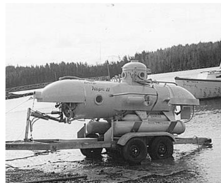
The two-man, 25' long Deep Hope II built by Hope Industries of PA in 1979 specifically for owner Jack Hope's salvage of the scuttled ketch Traveler III . Photo by Hope Industries (PA), published June 2010 in Fishermen's Voice .
